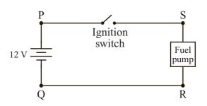
This fuel pump may have an internal short circuit. At which two points should an ohmmeter be connected to measure the resistance of the fuel pump?
